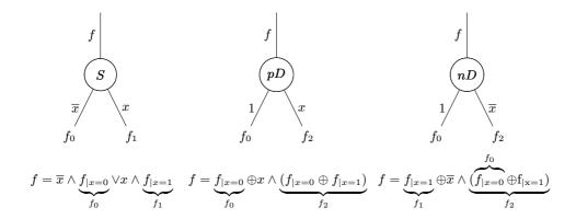
In [2] arithmetic BDD are considered for realization of BF systems — «Word level» —  $F(x_1, x_2, \ldots, x_n)$ . The lower circle of BDD based on the arithmetic Shennon decomposition, represents numerical values of the right column of the table of BF system validity; the lower circle of BDD based on the arithmetic positive Davio decomposition consists of coefficients from  $\mathbb Z$  polynoms received by generalization of a numerical normal form:
